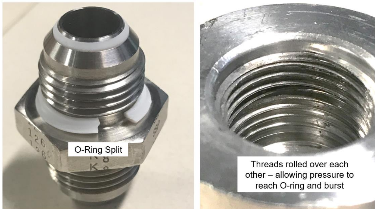
Figure 13. Burst test of test fixture 2.
