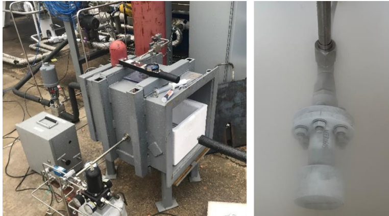
Figure 12. Cryogenic pressure cycle test set-up (Left), test fixture #3 installed in test set-up (Right).
