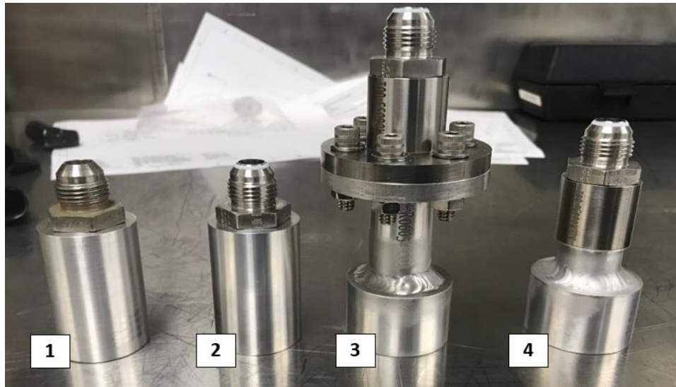
Figure 11. Test fixtures tested for aluminium to stainless-steel joints.
