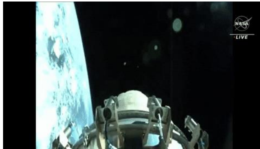
Successful inflation of the 6m diameter aeroshell
