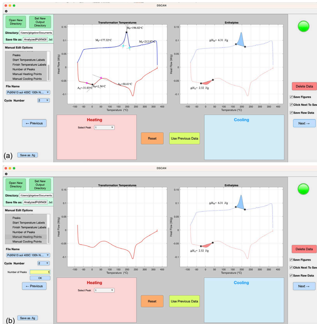
Figure 35.—Manual adjustment of parameters for a curve containing extraneous curvature in baseline horizontal portion of heating curve. (a) Initial automated analysis by DSCAN, which has identified this extraneous curvature as a peak. (b) Selection of Manual Heating Points option in Manual Edit Options menu box and input of “1” in Number of Peaks edit box. (c) Selection of points on Heating Transformation peak. (d) Automated fitting of the new peak.
