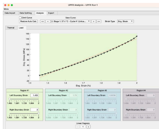
Figure 21.—Unloading segment of UPFR showing initial fit using a single region.
