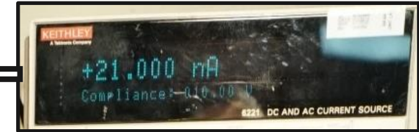
Laboratory current source (Keithley 6221)
