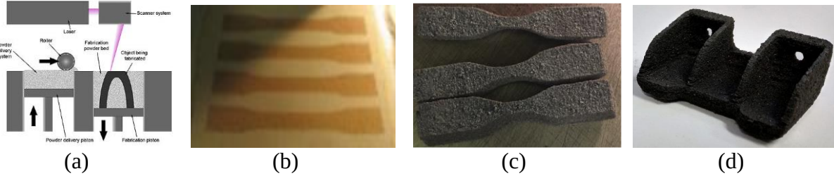
Figure 1. Laser sintering of RTM370 thermoset polyimide resin and composites
