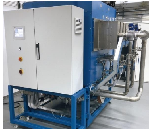
Figure 6: Largest membrane plant worldwide for the production of 14 kg O 2 /h. © Fraunhofer IKTS
