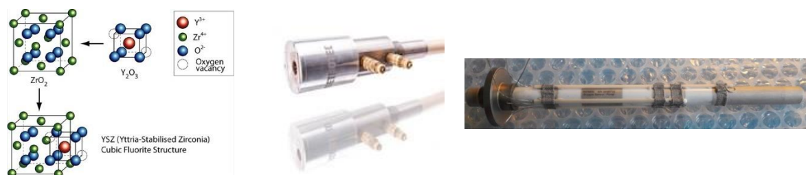
Figure 5: Left: Principle of oxygen ion conduction in yttria-stabilized zirconia, center: commercial oxygen sensor (Metrotec), right: combined oxygen pumping and sensing element for EML OCS on ISS (Airbus).
