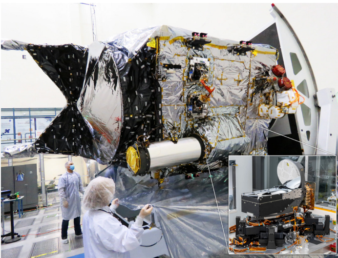
Figure 21: DSOC integrated on board Psyche and ready for launch.
