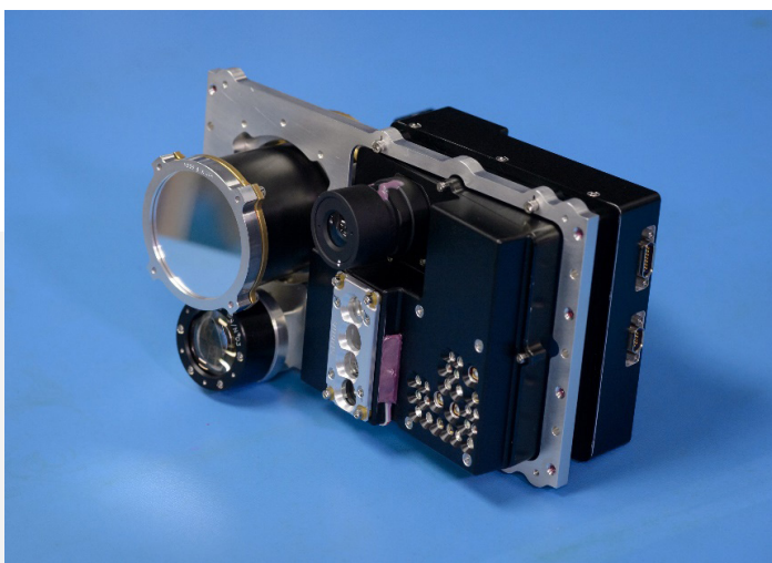
Figure 17: The Ames Imaging Module (black enclosure to right in photo above) integrate into the NIRVSS instrument. Credit: NASA Ames Research Center.
