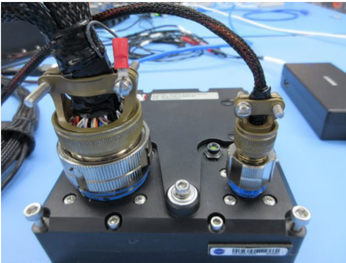
Figure 26: The flight S-A1760 Venus radiation-characterized Space AI GPGPU that provides high-performance computing capabilities that enable onboard integrated systems health management and autonomous operations.
