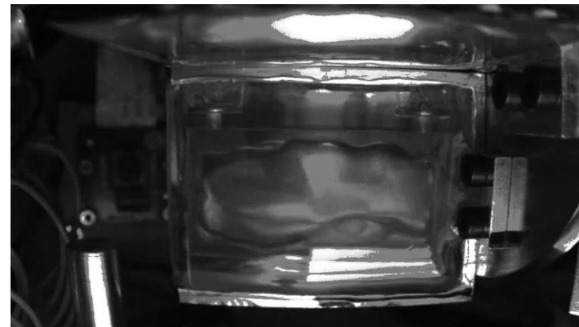
Above the Faraday Wave Threshold ( a_{sine} > a_c )
