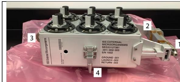
Figure 1: The sampling kit contains eight swab canisters in total (six on the top and two on the bottom). A reusable end effector (1) is used to remove and reinstall the swabs. The kit also contains a handrail (2), tether loop (3), and, bayonet probes(4) to allow easy manipulation during EVA.
