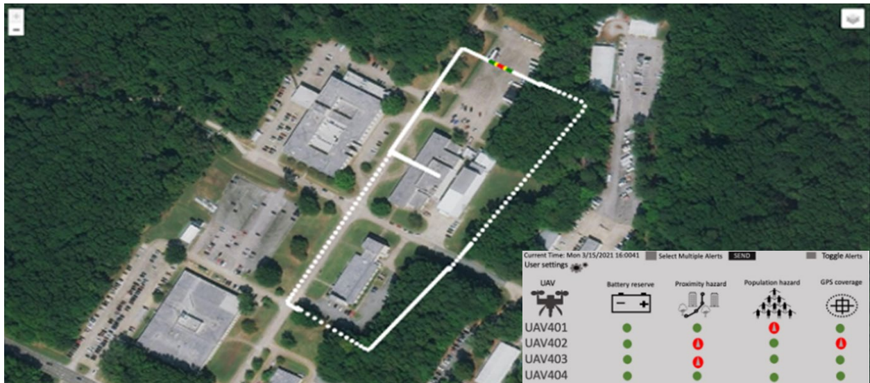
Fig. 2.2.3-2. The updated SDSP-CD GUI shows alerts for four flights in the table (inset) and in a map display. Population overflight hazards are shown on the map for one of the four flight paths. From [43].
