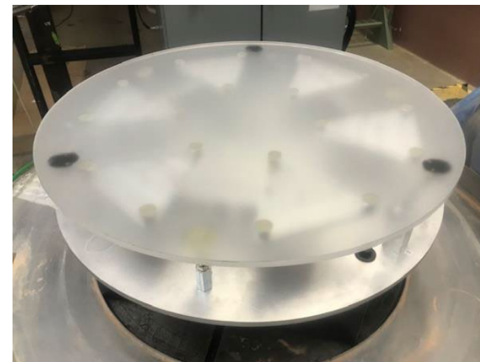
Mirror in Preparation for Cutting to Hexagon
