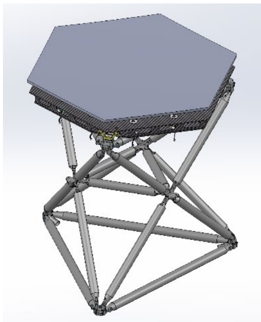
TriTruss supporting thin meniscus mirror
