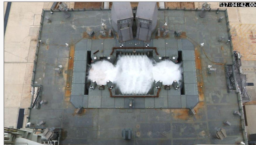
IOP/SS Water in Exhaust Holes
