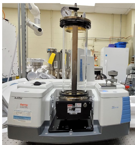
Figure 1. A glass-bodied long-path gas cell with variable optical pathlength capability, mounted on a Fourier transform infrared (FTIR) spectrometer.
