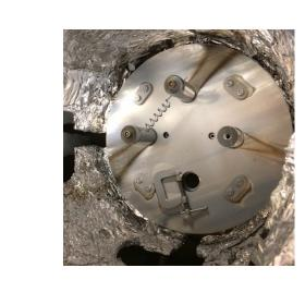
XeF<sub>2</sub> Gas feed components capable of continuous flow or pulsed flow.
