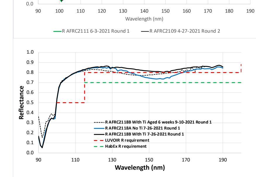
State-of-the-art reflectance performance of Al+LiF mirror coatings in the FUV spectral region.
