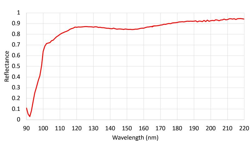
The FUV reflectance curve for a test witness (shown in the picture above) after the application of the Al+LiF by using the rPVD coating process.
