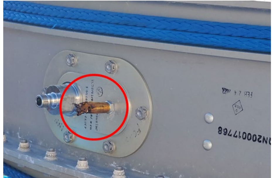
Kapton tape - note how pristine the surrounding area is compared to the tape
