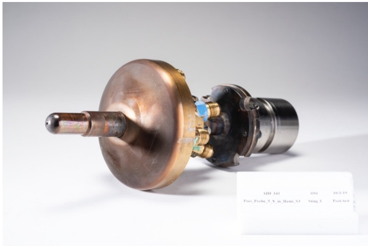
1.59-cm diameter hemisphere probes: pitot probe and Gardon gage calorimeter (TP3 15-inch nozzle, AHF 12-inch nozzle)
