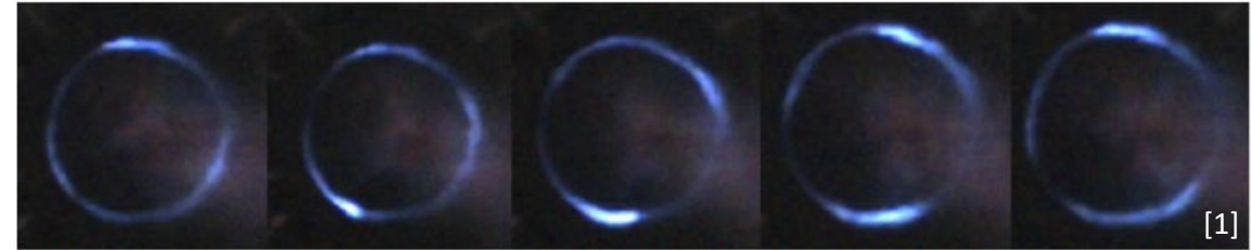
Fig 19. High speed images of liquid/liquid LOX/LCH4 co-rotating waves. Images show from left to right a frame-by-frame capture of the wave movement. [1]
