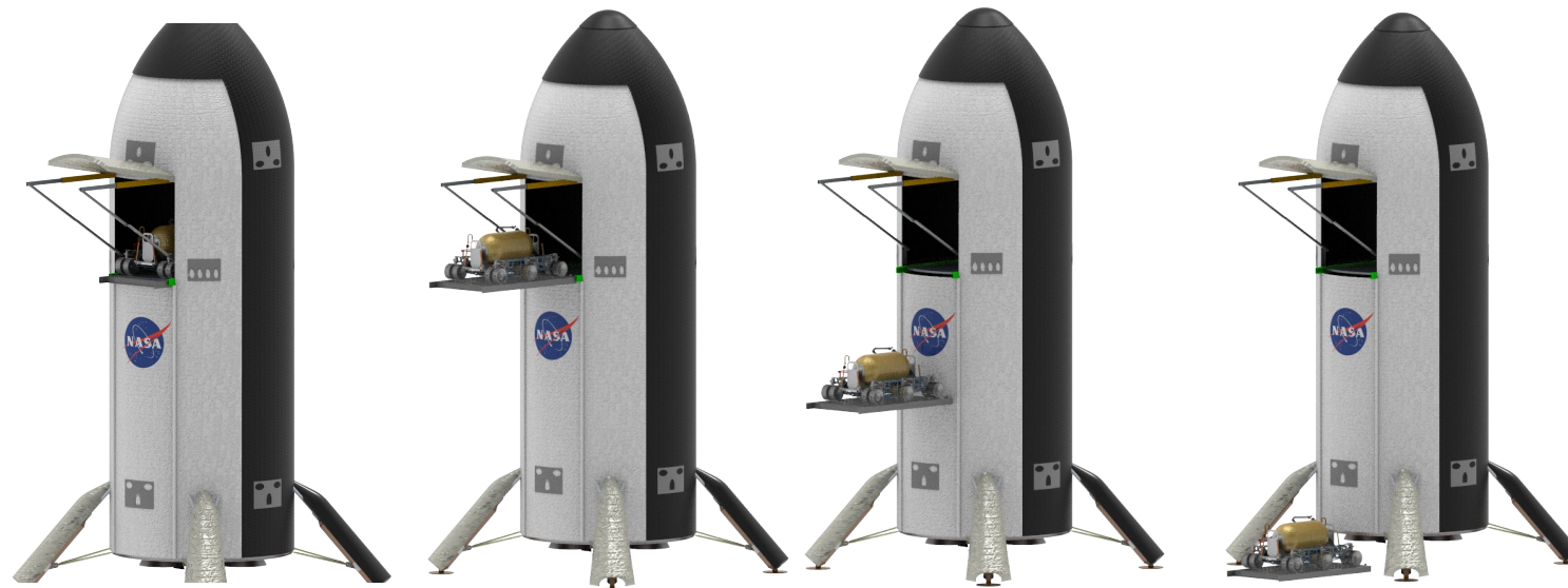
Surface Payload Deployment
