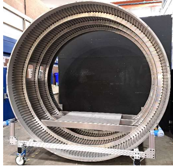
Figure 1. 3 m diameter, 1.524 m long fuselage manufacturing demonstration article with stiffeners.
