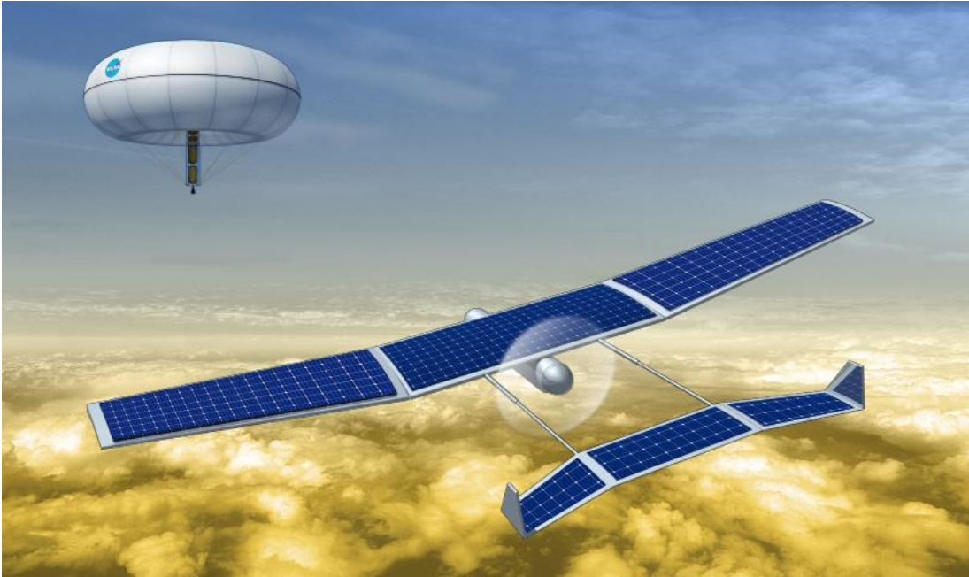
Figure 2: artist's conception of the airplane, now operating in solar-powered mode, approaching the balloon platform carrying the Venus launch vehicle.
