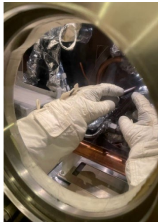
Figure 2. The DGB front hatch viewport with EMU gloves installed.
