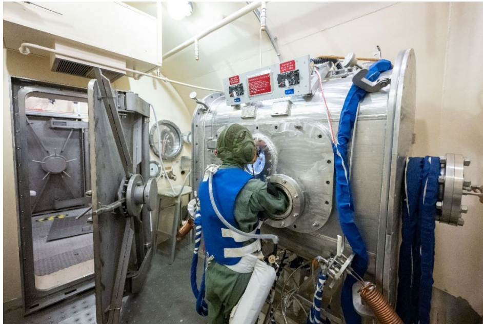
Figure 4. Test subject within the 11ft chamber and operating hardware with EMU gloves in the DGB.
