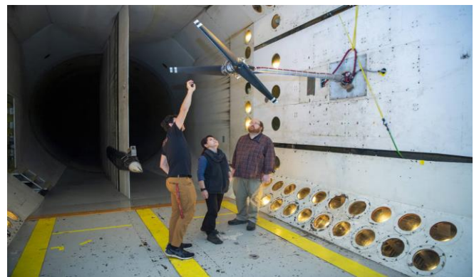
Figure 5. Fixed-Pitch Speed-Controlled Coaxial Rotor System in the NASA Langley Transonic Dynamics Tunnel, Ref. [50].
