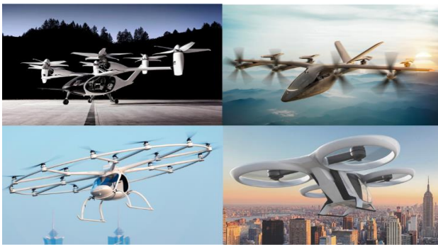
Figure 4. Example Multirotor Aircraft Under Development (starting top-left, then clockwise): Joby S4, Vertical Aerospace VX4, Airbus CityAirbus, and Volocopter VoloCity, Ref. [49].
