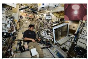
The JAXA ELF instrument on the International Space Station. Inset shows an image of a levitated sample. Courtesy of JAXA.
