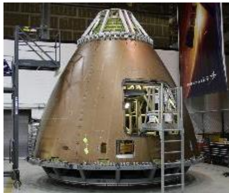
Artemis II Launch Abort System 0 Degree Ogive in Protoqual Testing
