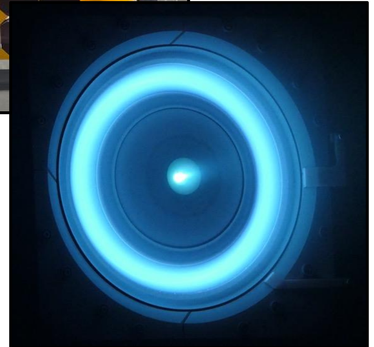
PPE 6-kilowatt SEP subsystem test
