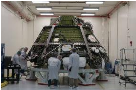
Crew Module ECLSS Bay Components Installed
