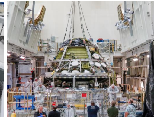
Integration of Crew and Service Modules for the Artemis II Orion Spacecraft Complete
