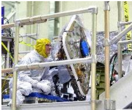
Artemis II Slide Hatch in Acceptance Testing
