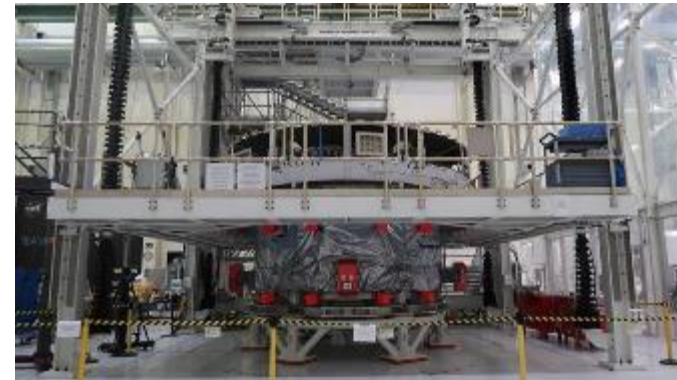
Crew Module Adapter and European Space Module Mate
