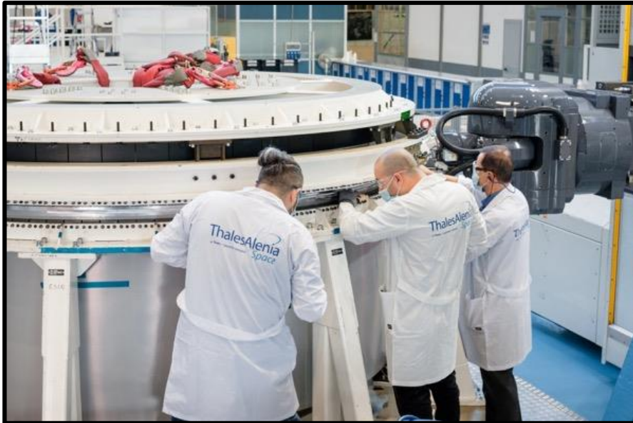
HALO primary structure assembly at Thales Alenia Space Italy (TASI)
