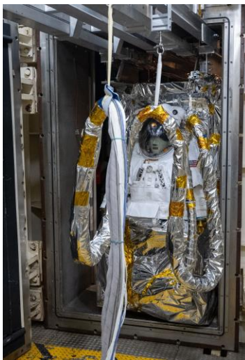
Figure 3. SxEMU Test Article Traversing into the Manlock.
