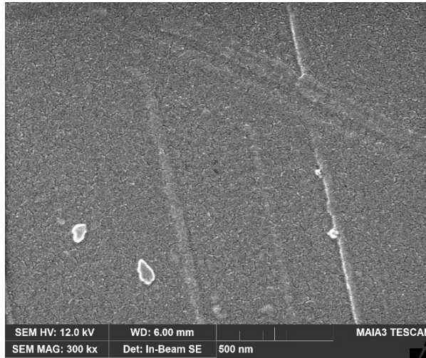
Figure 46. FESEM images the Kapton H layer of the M12Z-Z1 F AO Photo Monitor. (a) 200X at the exposed-protected border, (b) 300kX in the protected region, and (c) 300kX in the exposed region.
