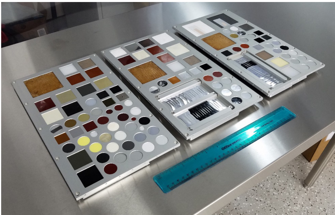
Figure 7. Pre-flight photograph of the MISSE-9 PCE-1 samples loaded into the MSC MS flight decks, from left to right: R2 MSC 3 (ram), W3 MSC 8 (wake), and Z3 MSC 5 (zenith).
