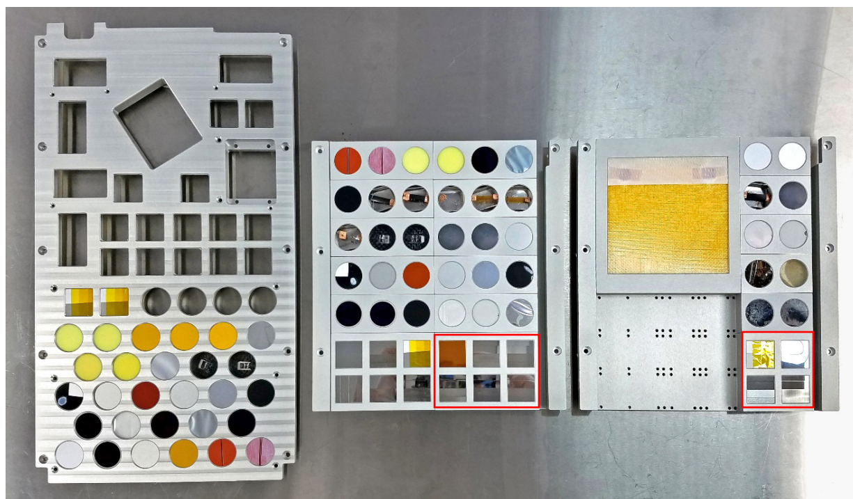
Figure 12. Pre-flight photograph of the MISSE-12 PCE-3 samples loaded into the MSC flight decks, from left to right: R2 MSC 4 SS (ram), W3 MSC 6 MS (wake), and Z1 MSC 18 MS (zenith). Samples in red boxes were moved to a different location on the deck prior to flight.
