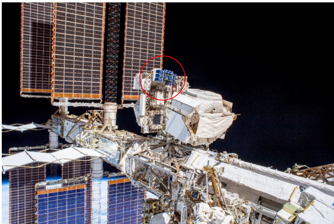
Figure 21. A view of the MISSE-FF on ELC-2 Site 3 as photographed during an EVA on November 15, 2019 (iss061e040917).
