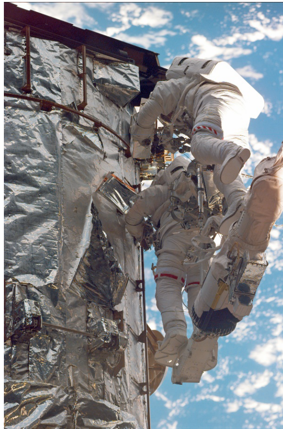
Figure 5. Large cracks in the outer layer of solar facing multilayer insulation (MLI) on the HST as observed during SM2 after 6.8 years of space exposure. 12
