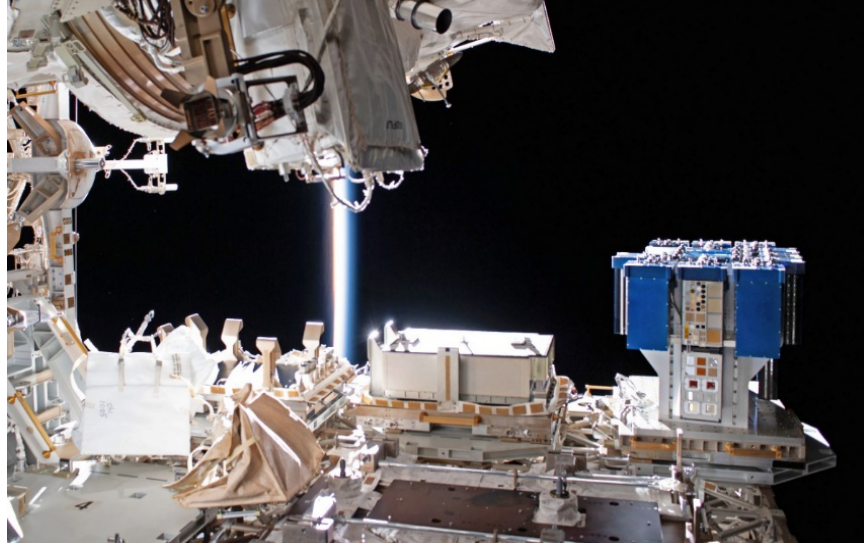
Figure 29. The wake side of the MISSE-FF with the MISSE-10 PCE-2 and MISSE-12 PCE-3 MSCs as photographed on January 25, 2020 during an EVA. The MSCs are closed, except for the central wake MSC which is open (iss061e143021).
