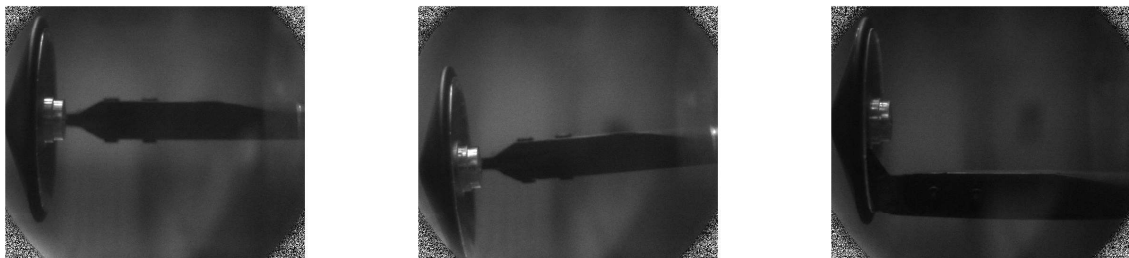
Figure 9. View from the PLIF camera (equipped with a 45 mm UV lens) in long-exposure mode for the three model configurations: (a) \alpha = 0^\circ , \beta = 0^\circ , (a) \alpha = -5^\circ , \beta = 0^\circ , (a) \alpha = 0^\circ , \beta = 90^\circ .
