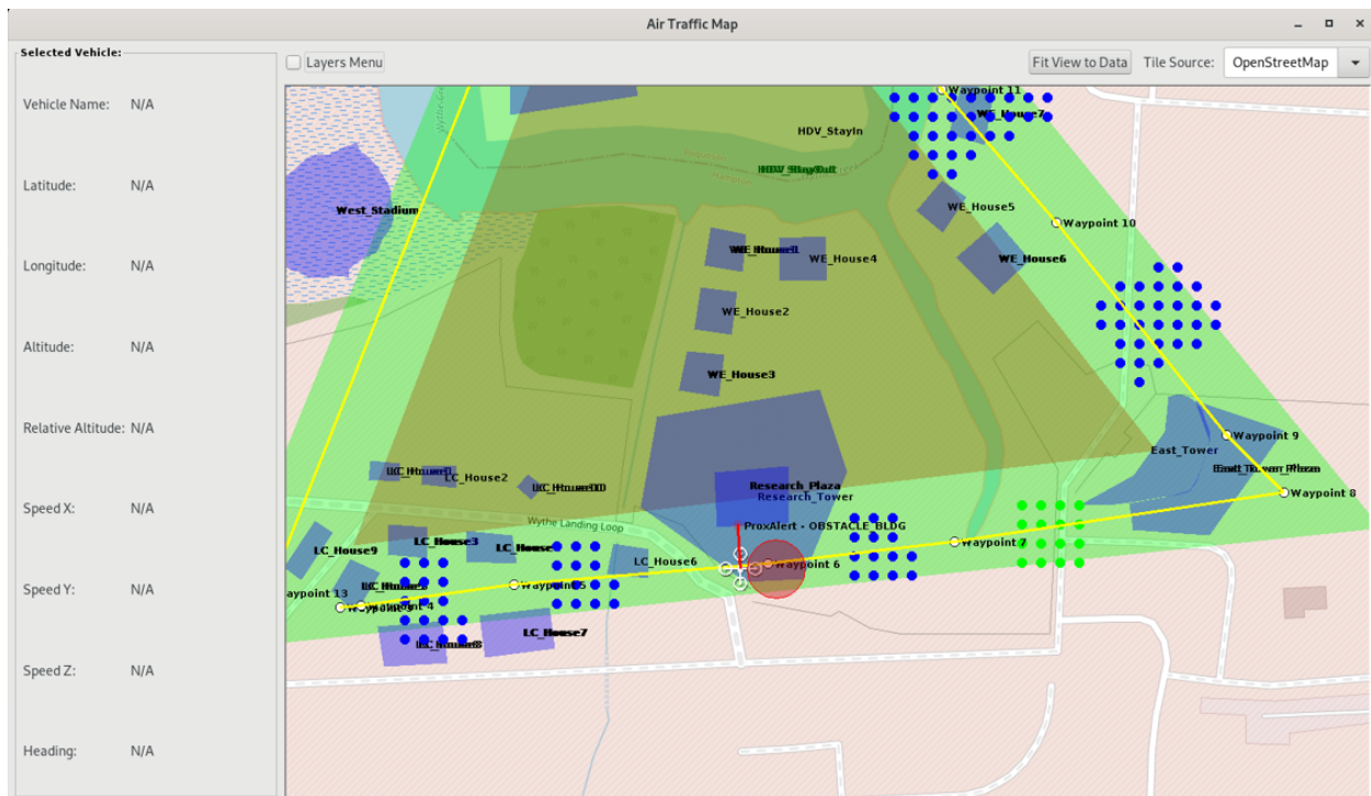
Figure 8. —PtT function tested onboard an octocopter flying over CERTAIN fictional city. The flight route is the yellow line, the vehicle is the white symbol toward the bottom of the image, and the red line extending from the vehicle to a building shows a proximity violation. Although PtT produces an alert for every trajectory point that violates the client-specified thresholds, only a single red line depicting the nearest alert is shown on this image to save bandwidth. (NASA image. Maps Data: Open Street Maps)
