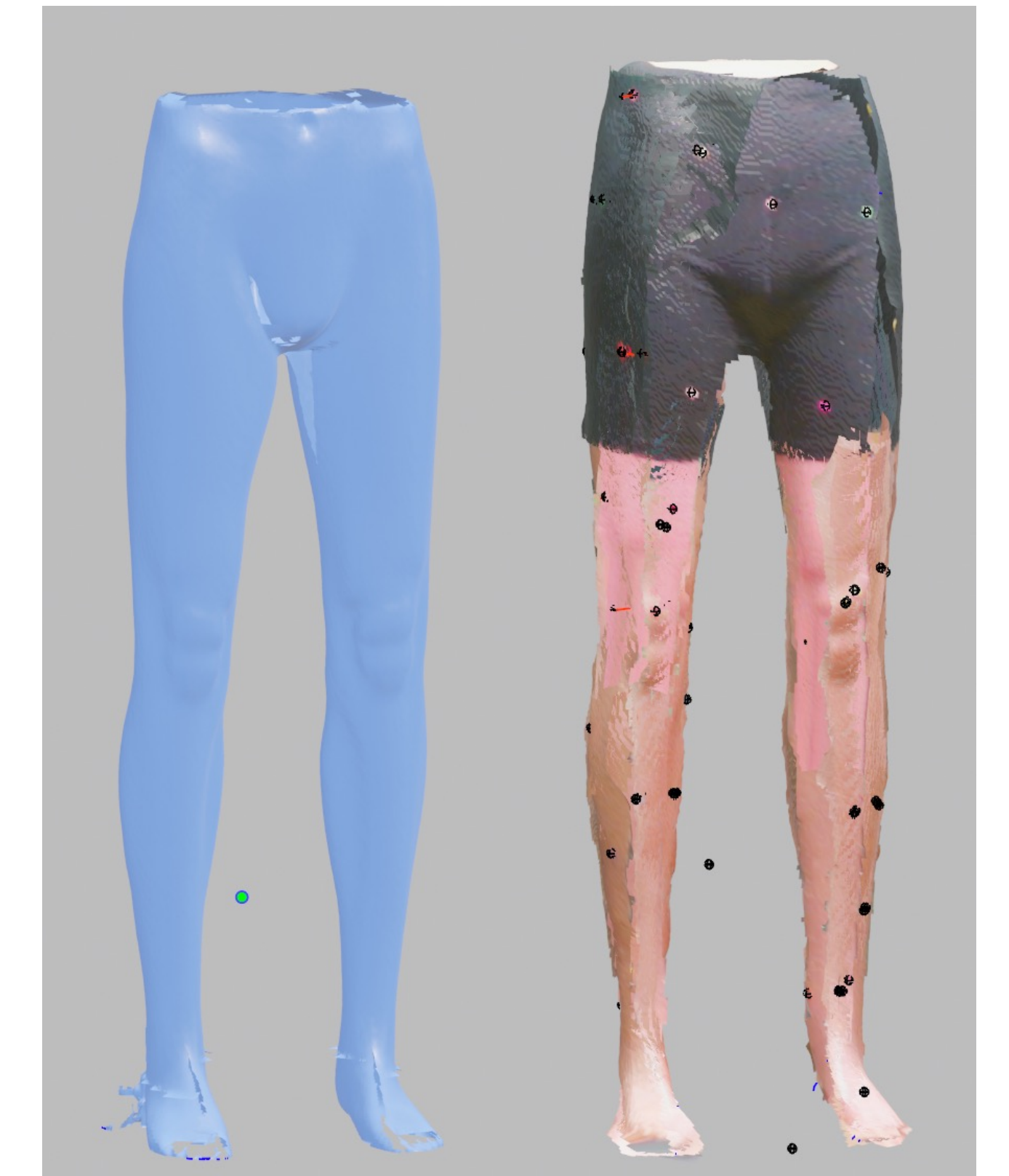
Preliminary scans: reference (HumanSolutions Vitus) vs. proposed hardware (Intel RealSense)
