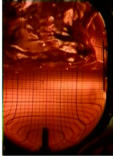
Sequence A (9.6 s): elongating of the ullage along the central axis creates “apple core” shape
