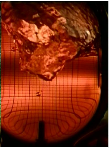
Sequence C (124.3 s): rotation of the ullage results in elongated asymmetrical ullage shape
