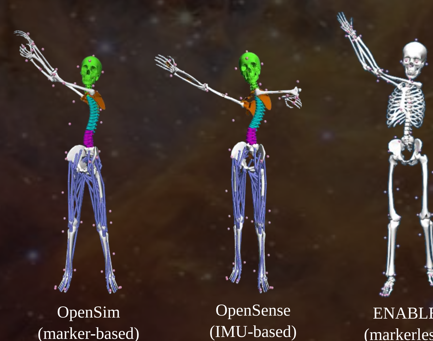
Figure 4. Kinematic results from marker-based, IMU-based, and markerless video-based pipelines for a subject performing a Chop exercise.
