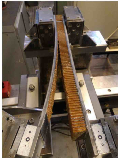
(c). Typical crack opening for a DCB-UBM specimen. Id: 8-7-1-L-T-U-N-F-05-02.
