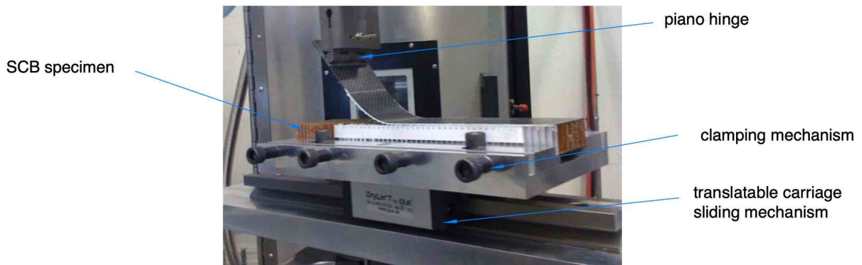
(b). Detail of test fixture.
