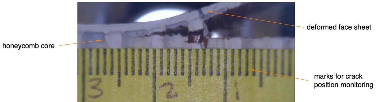
(b). Stabilized disbond location grown from machined starter crack for the baseline tests.
