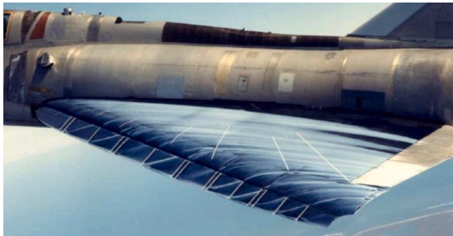
Fig. 35. Vortex tearing, F-106B VFFE. M \sim 0.3 , Re_{c_{ref}} \sim 40 \times 10^6 , \alpha = 10^\circ , \delta_f = 40^\circ . Brandon et al. [50], 2003.
