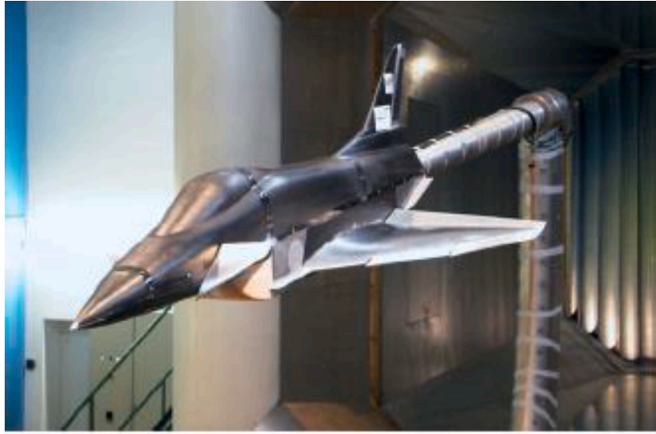
Fig. 92. X-31 model. \Lambda_{le} = 57^\circ/45^\circ . Schütte et al. [175], 2012.
