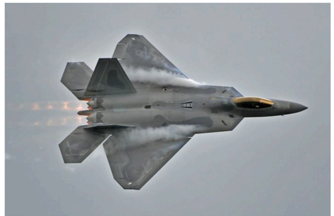
Fig. 6. Maneuver vortex lift. Contemporary design. F-22, first flight in September 1997. [Photo: copyright Russell F Spencer, www.russellspencer.com , reprinted with permission].
