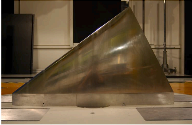
Fig. 58. Diamond wing model, \Lambda_{le} = 53^\circ . Luckring et al. [107], 2016.
