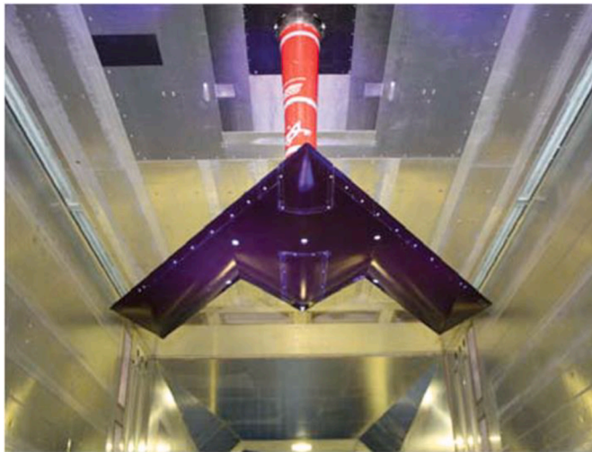
Fig. 83. SACCON low-speed wind-tunnel model. Cummings and Schütte [158], 2012.
