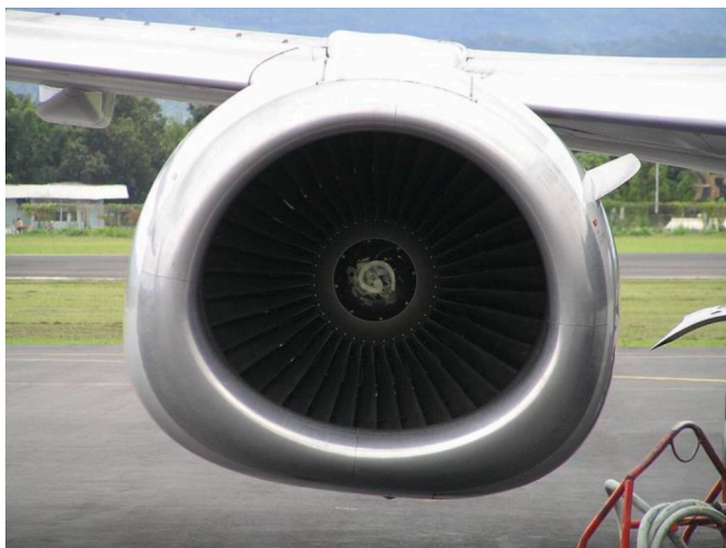
Fig. 14. High-bypass-ratio engine with nacelle strake. Boeing 737-400. [Photo: Stackexchange, reprinted under Creative Commons License].
