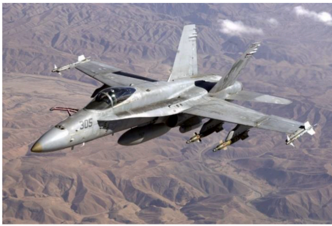
Fig. 4. Leading-Edge Extension, F-18C/D. F-18A/B, first flight in November of 1978. [USN, public domain].
