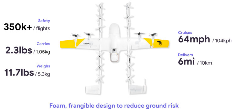
Figure 5. Wing Performance Parameters
