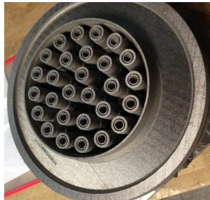
28-element Inconel® 625 fuel injector built using a laser powder bed fusion (L-PBF) process
