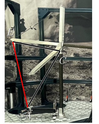
(a) Cable A does not rest against pulley D when \theta_1 \geq \theta_1^* .
