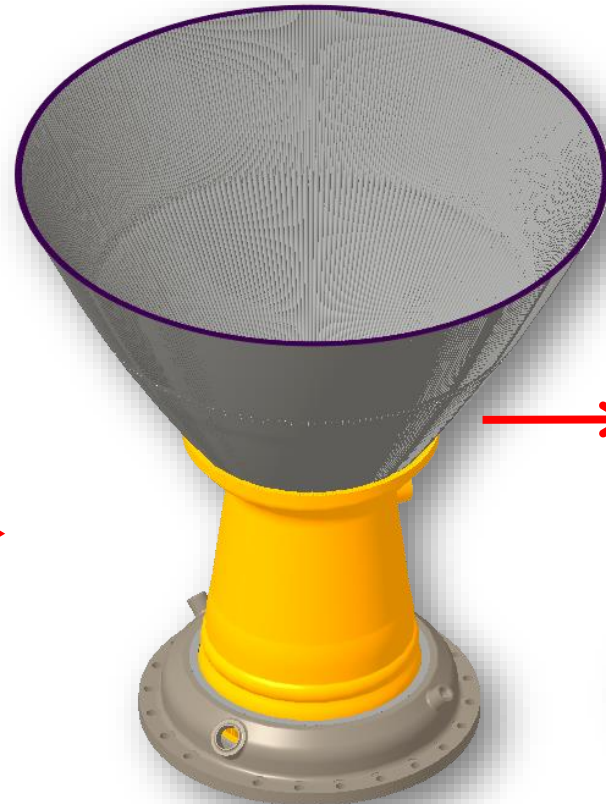
Laser Powder DED of Regen- nozzle directly on chamber
