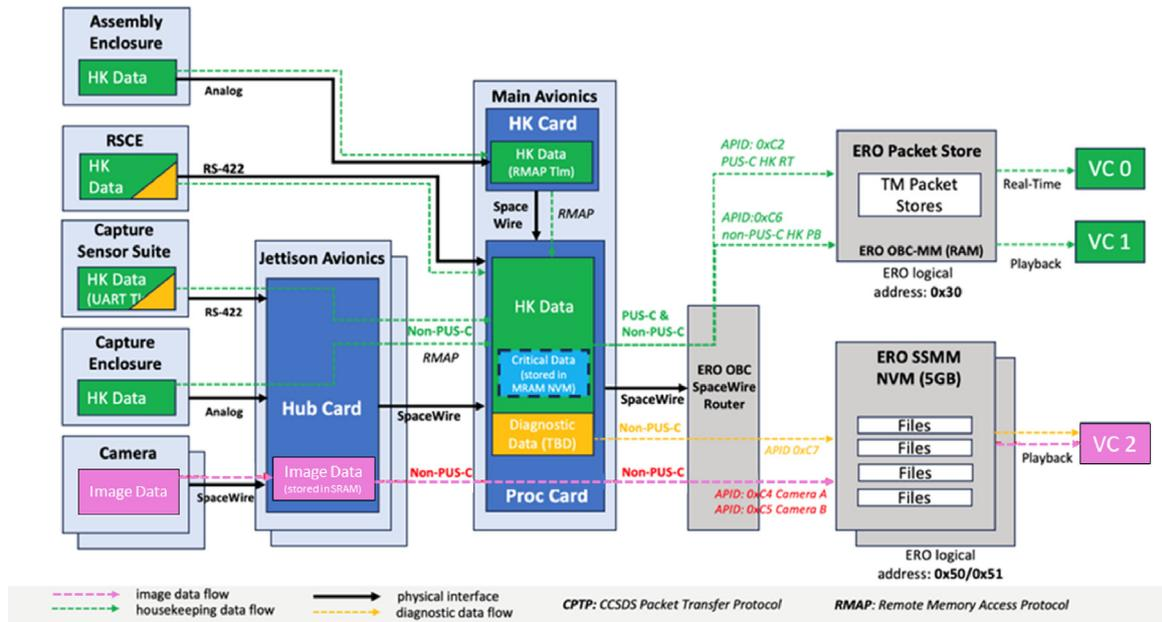
Fig. 15. CCRS on-board data flow to ERO.
