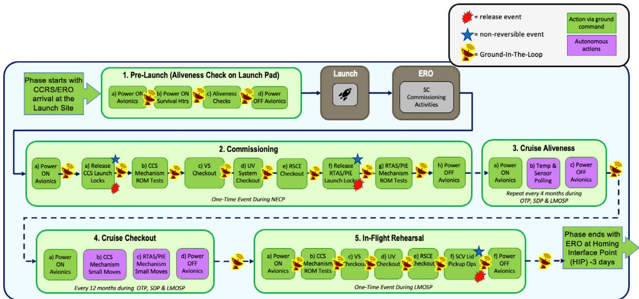
Fig. 19. CCRS workflow during LCOT phase. LCOT phase has two irreversible events and three release events.
