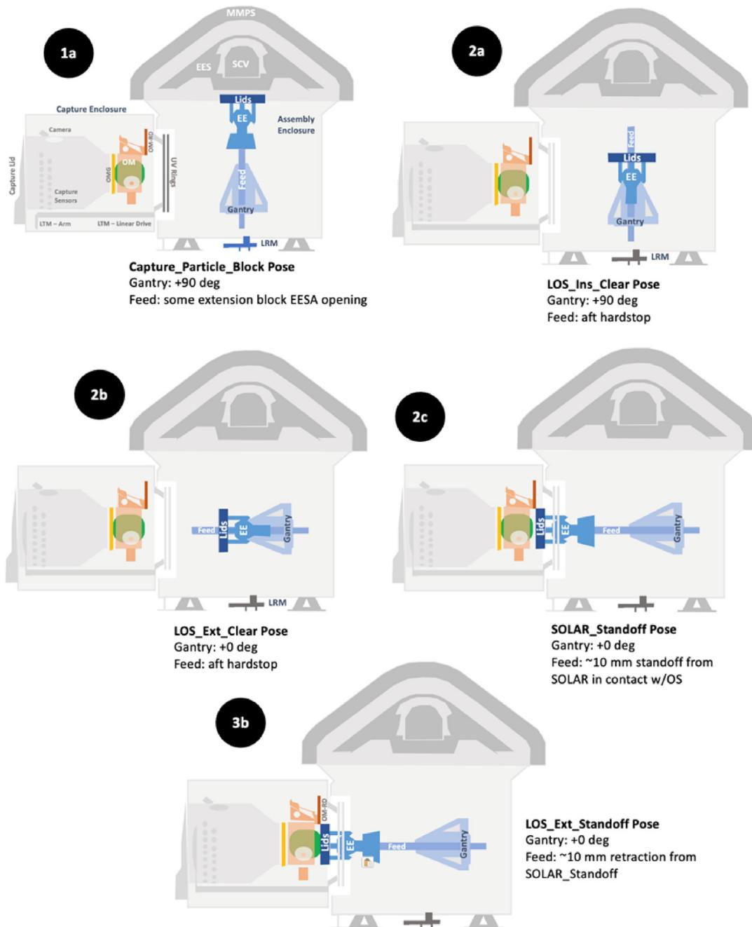
Fig. 29. OS pickup subphase: Assembly mechanism (gantry) poses moving the OS lid assembly from the particle closeout position to the standoff position.
