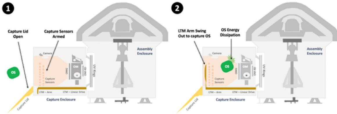
Fig. 24. Capture subphase configurations before and after OS entry into capture cone. Kinetic energy imparted from the OS is dissipated via collisions in the capture cone.
