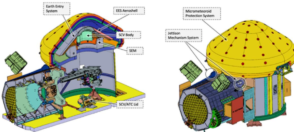
**Fig. 12.** Model of the micrometeoroid enclosure components.
