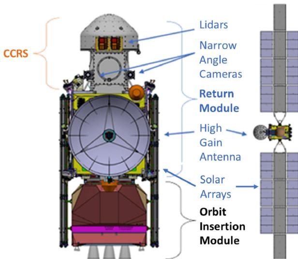
Fig. 5. Stowed and deployed ERO spacecraft configurations.
