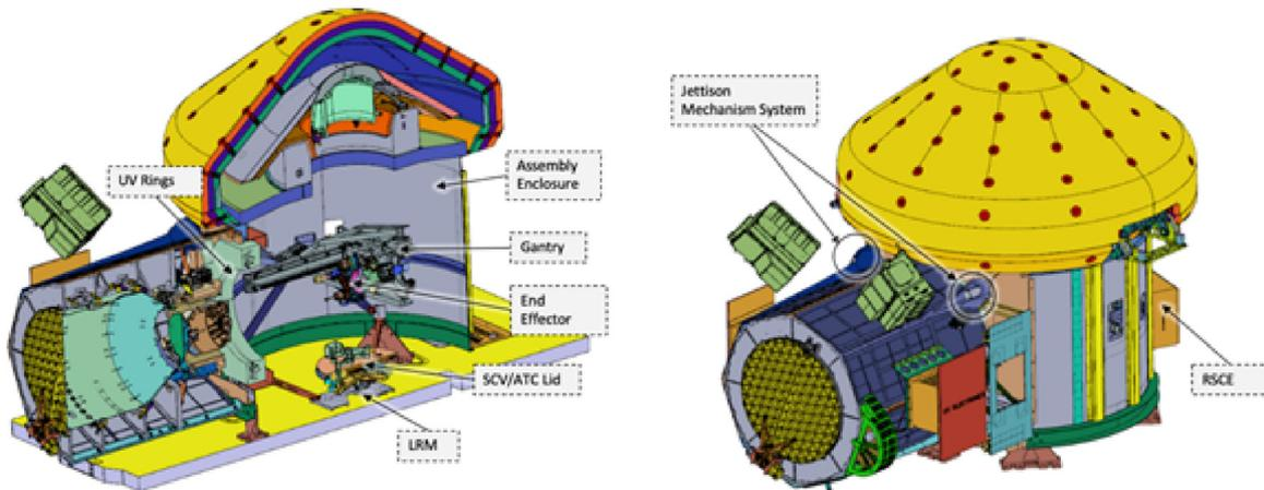
**Fig. 11.** Model of the assembly enclosure components.
