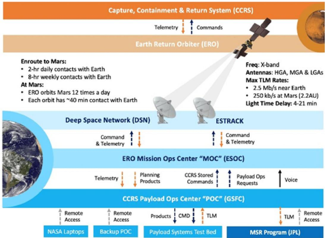
Fig. 16. CCRS ground system architecture through DSN and ESTRACK.
