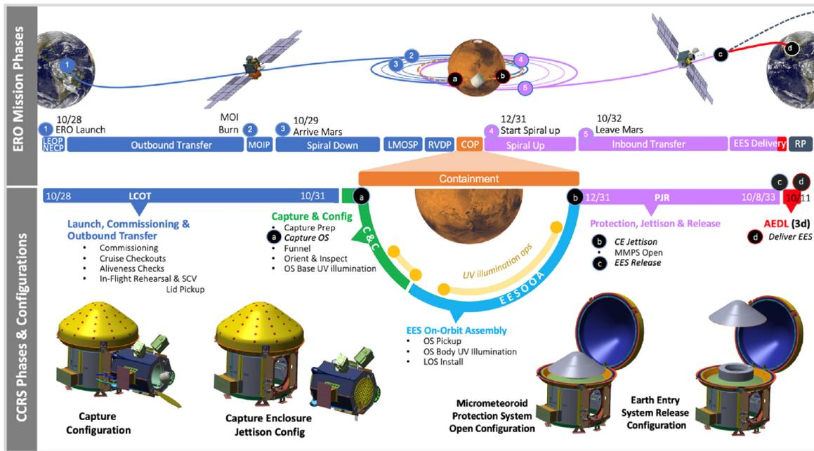
Fig. 4. Planned CCRS and ERO phases with key events and CCRS configurations.
