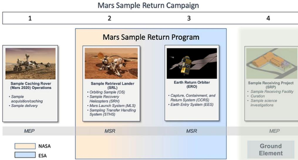
Fig. 1. Planned MSR campaign elements: Mars 2020 in its operational phase, SRL and ERO in their design phase as part of the MSR Program, and the SRP in its formulation phase.
