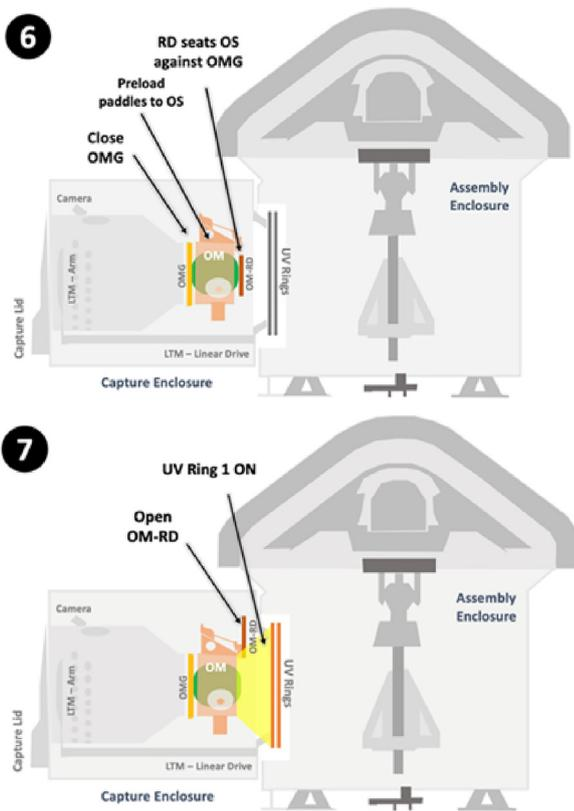
Fig. 27. C&C OS base illumination subphase configurations. The C&C phase ends with the completion of the UV illumination of the OS Base and the OM-RD Open.
