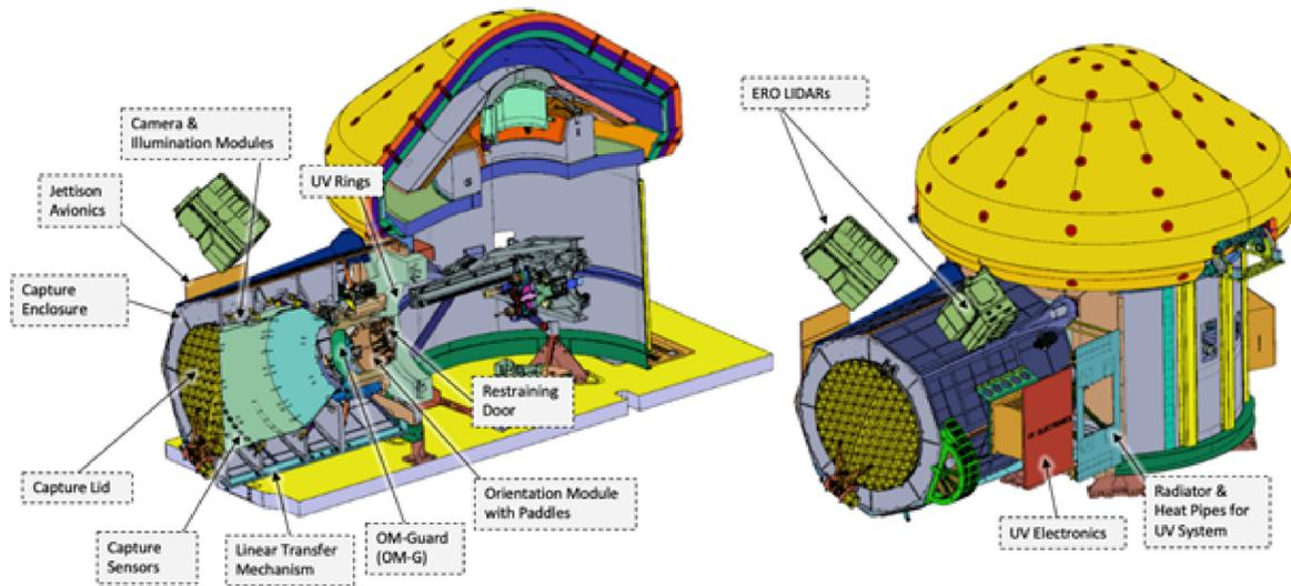
Fig. 10. Model of the capture enclosure components.
