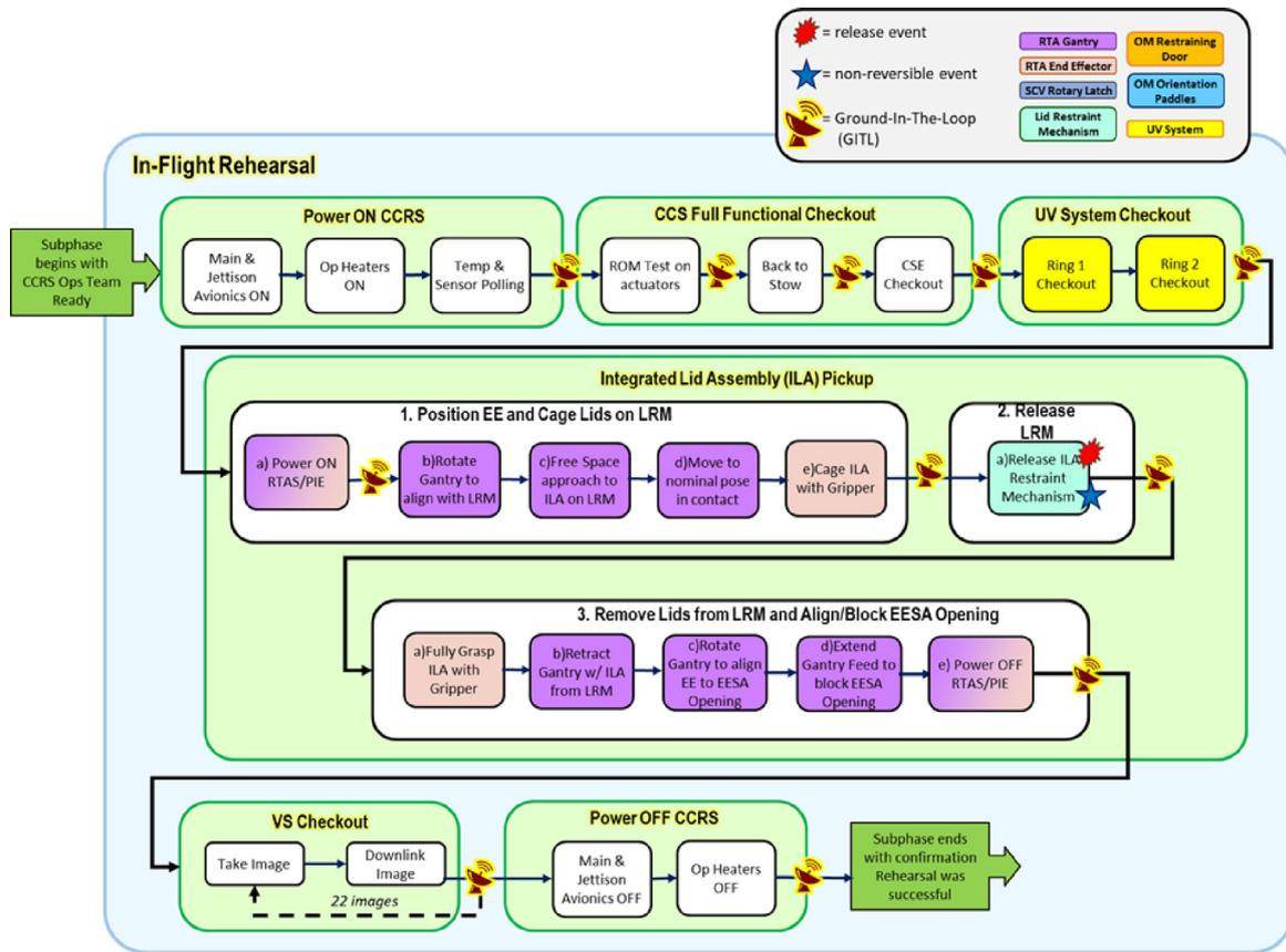
Fig. 20. CCRS activity workflow during in-flight rehearsal of LCOT.
