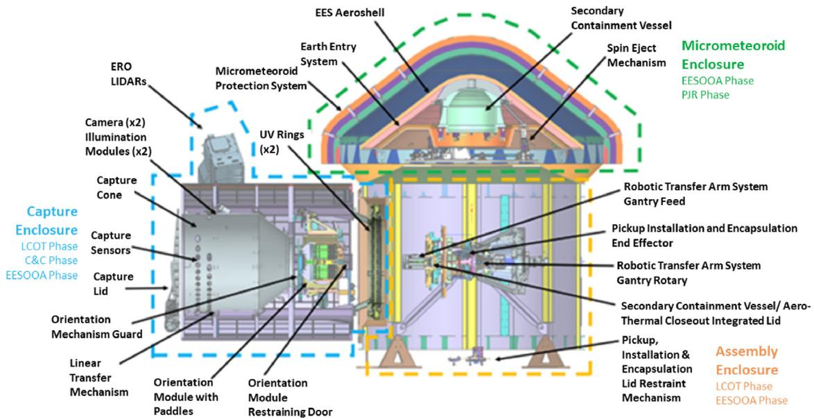
Fig. 9. CCRS payload element displaying the three CCRS element modules and major system components. The overall dimensions of CCRS are approximately 3.4 m × 0.5 m × 2 m.
