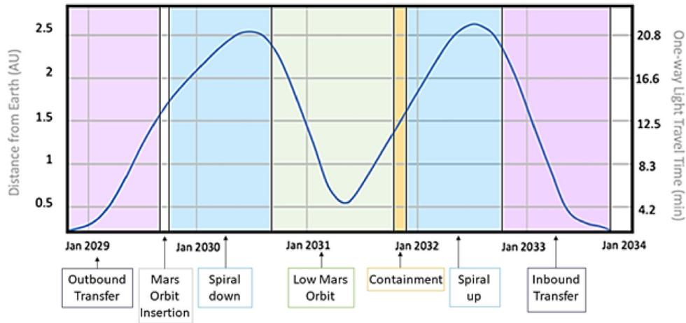
Fig. 7. ERO-CCRS distance from Earth and light time delays during SRL relay for a 2028 Launch. The longest communication delays occur in the summers of 2030 and 2032.
