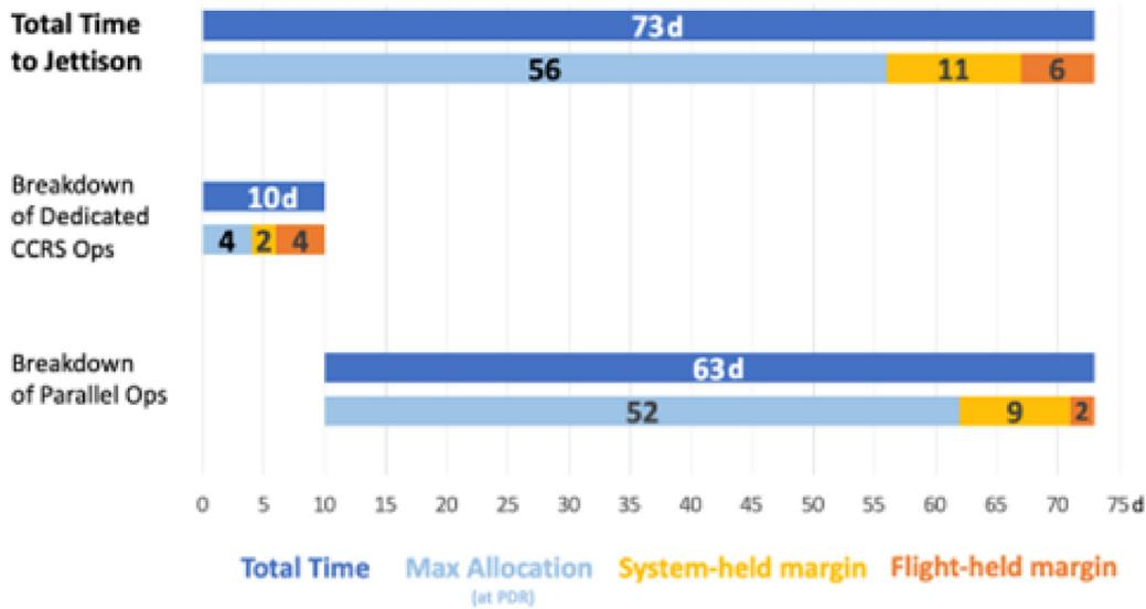
Fig. 17. Jettison timeline allocation of CCRS and ERO with system and flight margins.
