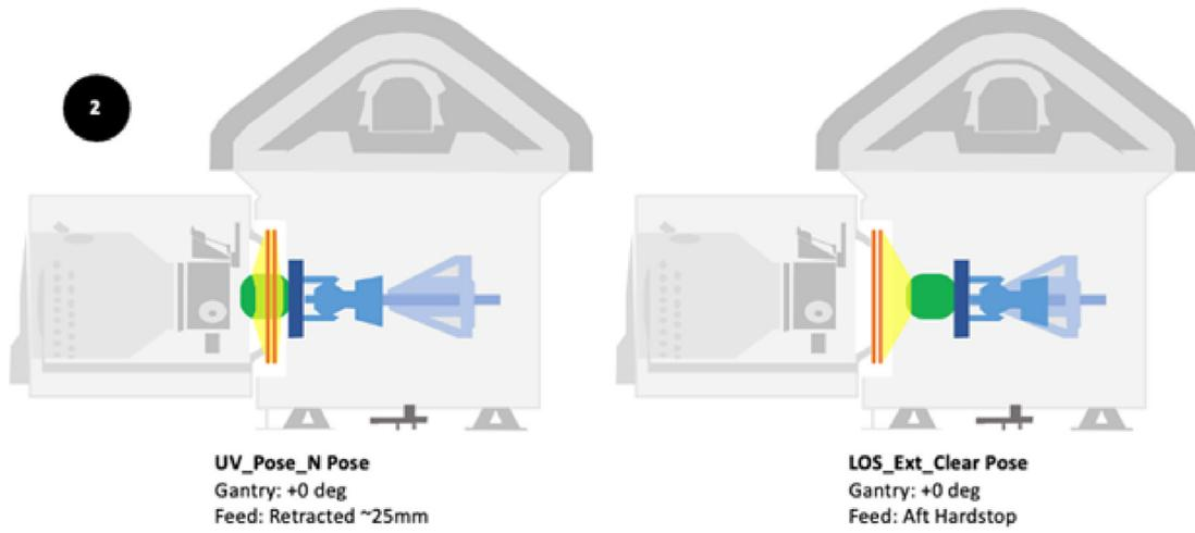
Fig. 30. UV illumination subphase gantry poses as it moves the OS through the UV ring in 25-mm steps.
