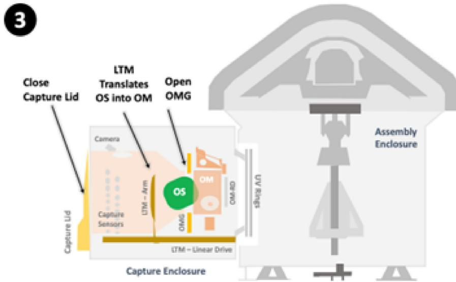
Fig. 25. Funneling subphase configuration with the translating LTM after the initial OS energy dissipation.
