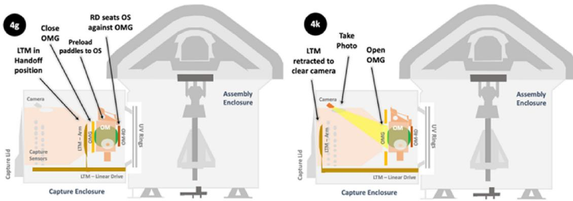
Fig. 26. C&C orientation and inspection subphase configurations. Proper OS orientation is checked using a camera at the front of the capture cone.
