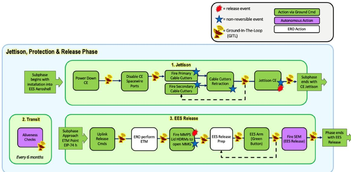
Fig. 33. CCRS workflow in PJR phase. PJR phase has five irreversible and release events.
