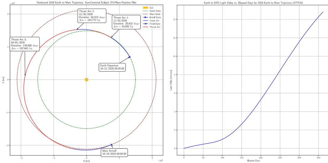
Fig. 6. The 302-day ERO-CCRS Outbound Trajectory from Earth-to-Mars and the Light Time Delay for a 2028 Launch.
