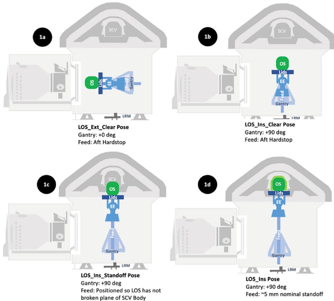
Fig. 31. Gantry poses as it positions the LOS for installation in the EES.
