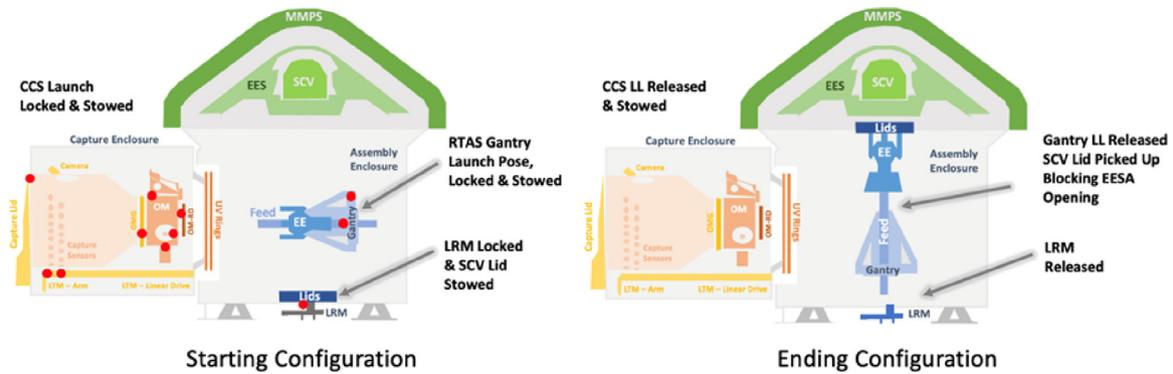
Fig. 18. LCOT phase starting configuration during launch and ending configuration approaching Mars.
