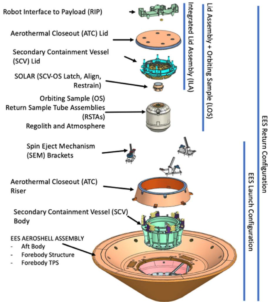
Fig. 37. Earth Entry System (EES) components with the assembled OS inside.
