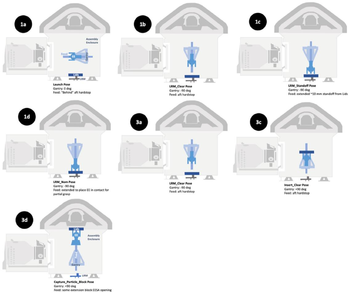
Fig. 21. Integrated lid pickup gantry poses to protect EES from loose debris during capture.
