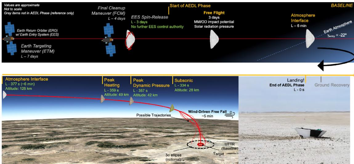
Fig. 36. AEDL phase timeline of events. EES is in free flight for three days before reaching Earth atmosphere interface.
