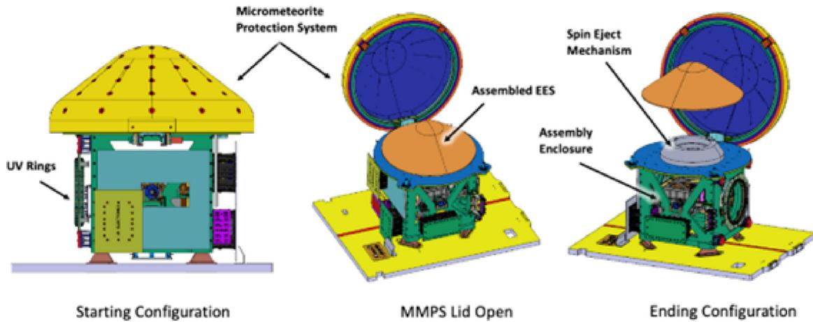
Fig. 35. Configurations for the EES release. The major mechanism operations for release include opening the micrometeoroid lid, and initializing the spin eject mechanism.
