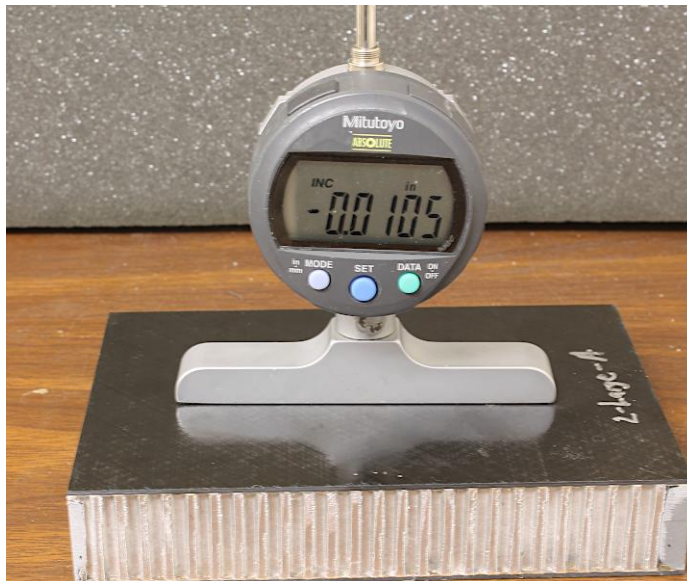
Figure 5. Dial gage used in this study to measure dent depths of impacted specimens.
