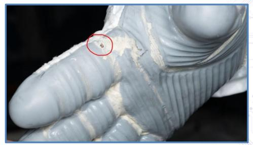
FY22: ISS demo of an AI/ML prototype Astronaut glove inspection model that performed diagnostics & generated a GO/NO-GO recommendation in 45 seconds on the glove condition, a process that normally is performed by a group of people taking multiple days.
