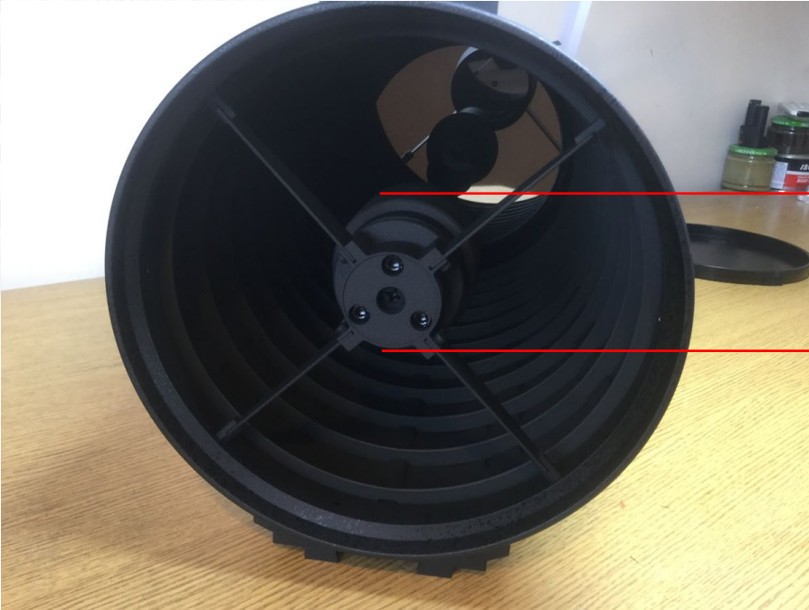
Schmidt-Cassegrain secondary mirror blockage
