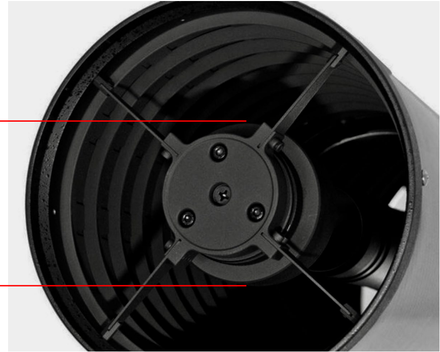
Ritchey-Chretien secondary mirror blockage is larger due to hyperbolic, vs spherical ground mirrors (will need to factor this for a clear aperture calculation).
