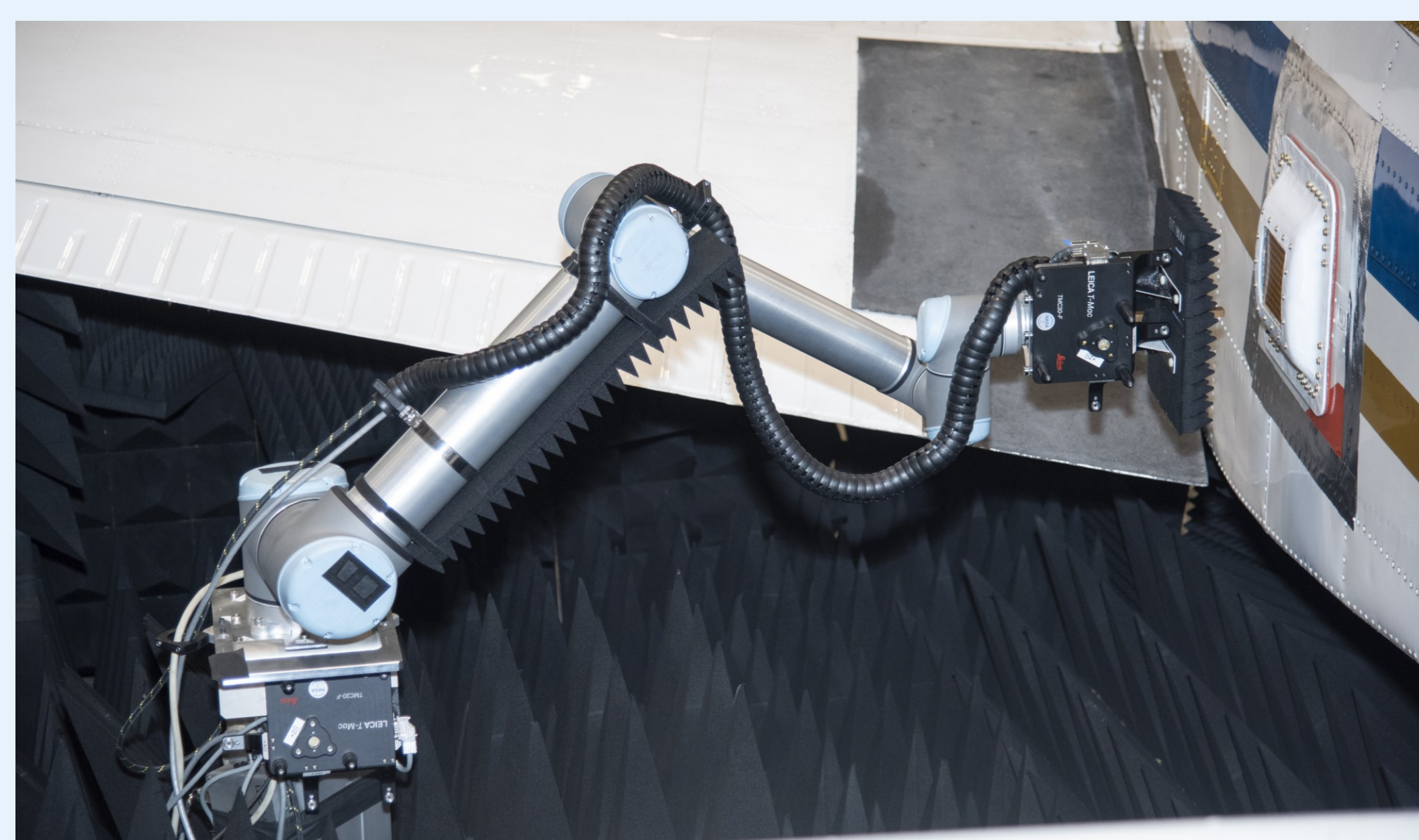
Antenna Calibration using the Portable Laser-Guided Robotic Metrology (PLGRM) System
