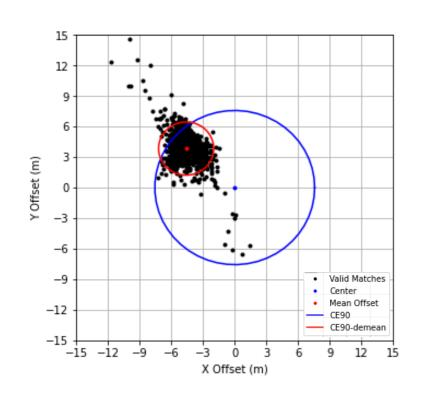
**CE90-demean:** CE90 but with the offset bias of the reference image removed. It is similar to a precision measurement of the target image.
