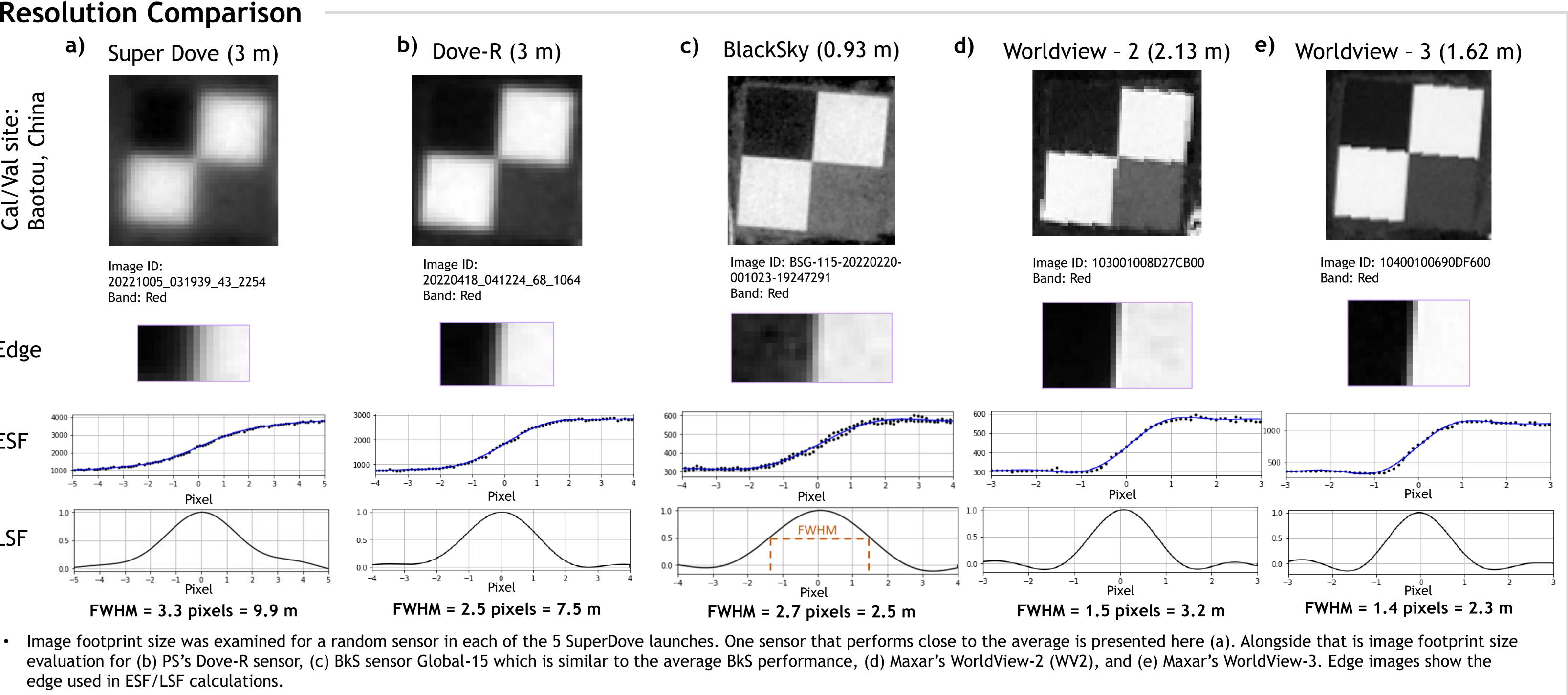
• When FWHM > gridded image pixel size, over-sampling occurs. When the FWHM/pixel-size ratio > 2, aggregation may be performed to reduce data volume and to increase SNR (signal noise ratio).
