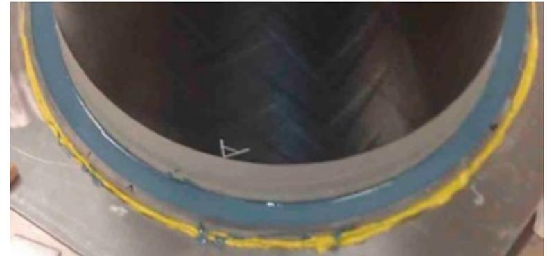
**Epoxy potting compound cast on shell ends to prevent brooming**
