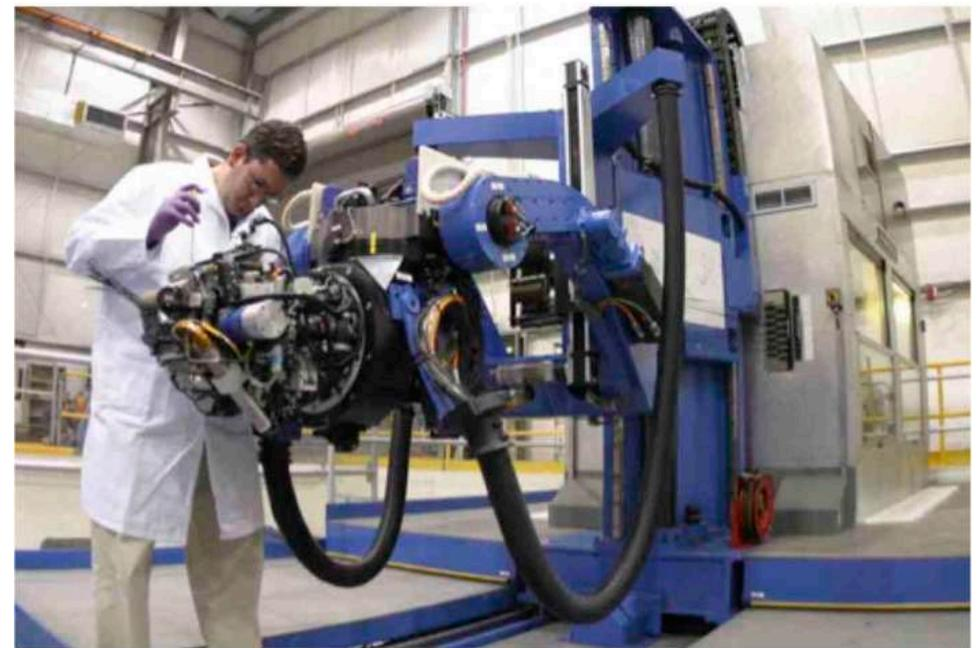
**Fiber placement system** has minimum steering radius => manufacturing constraint
