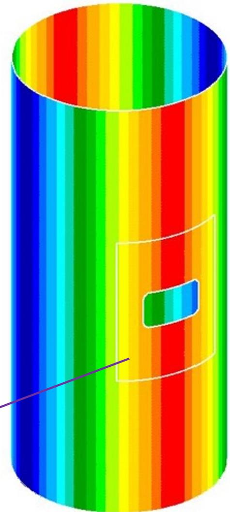
**Steered ply 3 fiber orientation angles**
