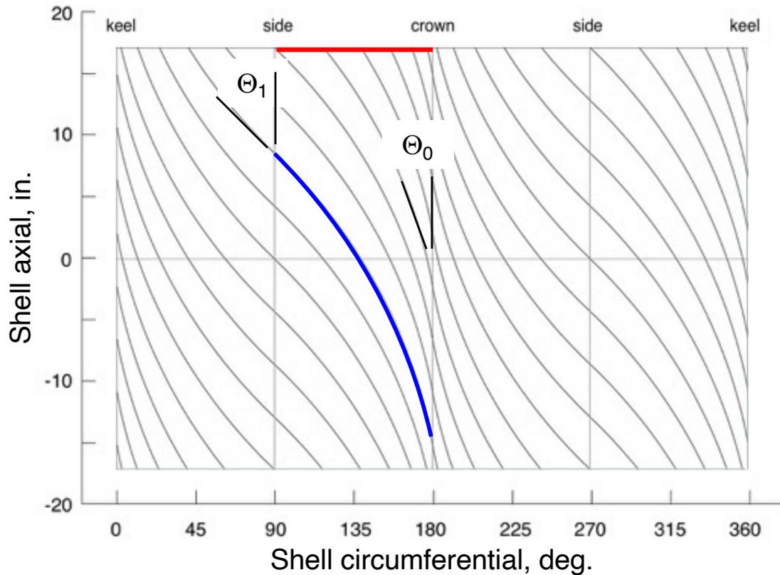
Continuous fiber angle variation from  $\Theta_0 = 10$  deg. on the shell crown/keel, to  $\Theta_1 = 45$  deg. on shell sides
