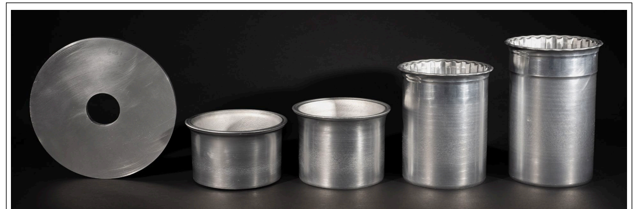
Forming Blank 8-Inch Diameter
