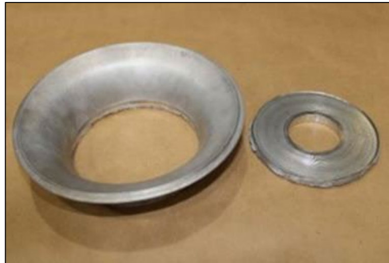
Premature fracture during forming
