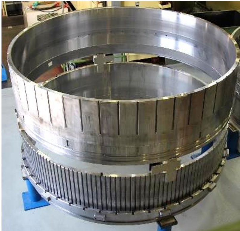
Two 10-ft. diameter ISC grooved mandrels
