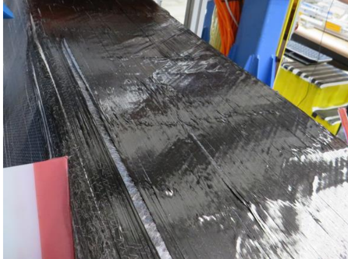
Figure 14: NCF Stitching Melted before Veil softened resulting in Fiber Distortion
