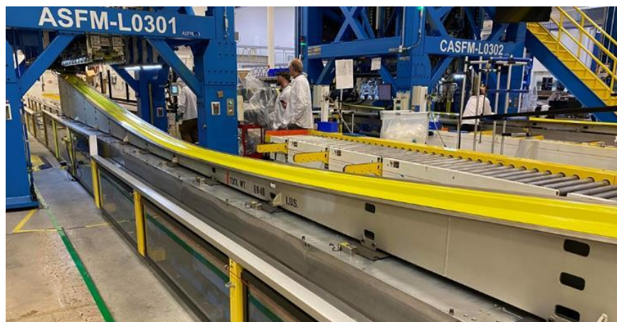
Figure 1: Automated Stiffener Forming Machine (ASF) Used for Production Thermoset Stringers
