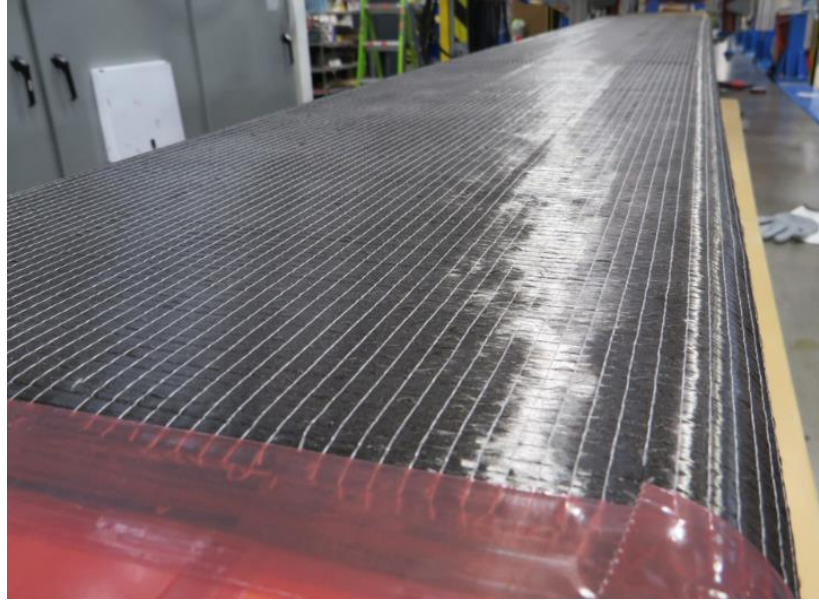
Figure 11: Teijin Biax NCF Showing Excellent Conformance to the Radius
