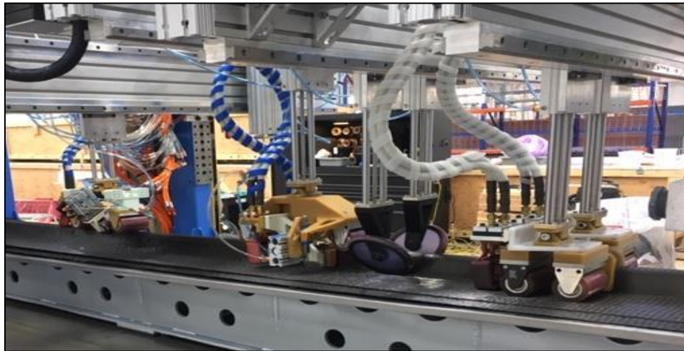
Figure 3: ASF Progressive Forming of an NCF Omega Stringer
