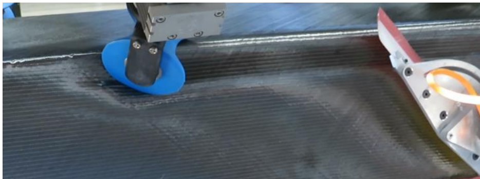
Figure 10: ASFM Forming a Biaxial NCF on a C-Channel
