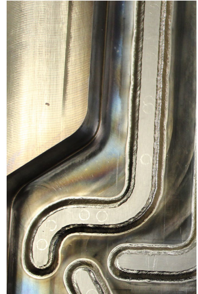
Weld track six imaged after electron beam welding
