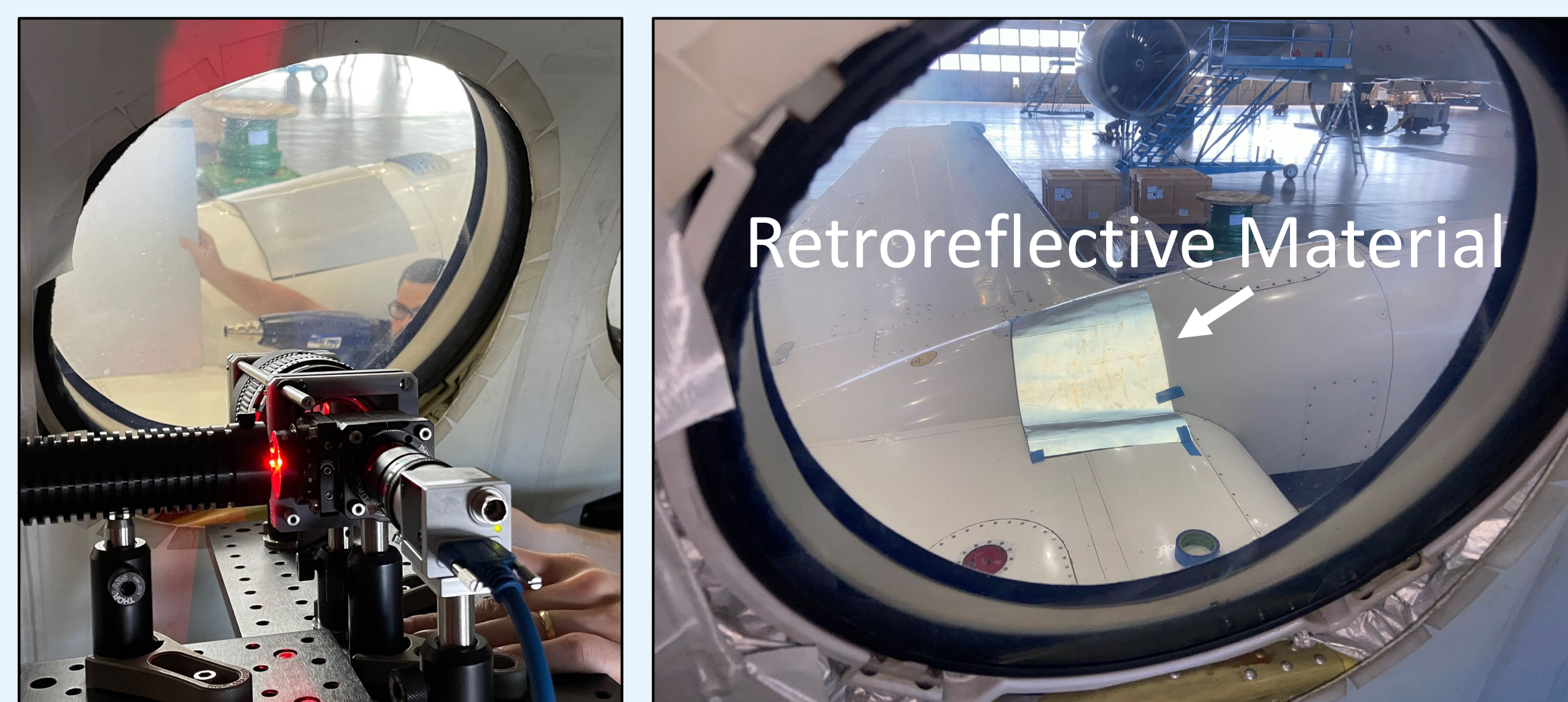
SAFS installed inside Beechcraft B200 King Air, with curved retroreflective material on engine cowling
