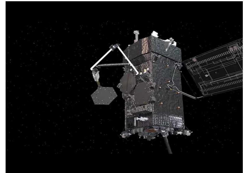
Space Infrastructure Dexterous Robot (SPIDER) in the OSAM-1 spacecraft
