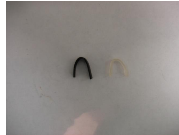
Programming (Deformation), T > T_g
