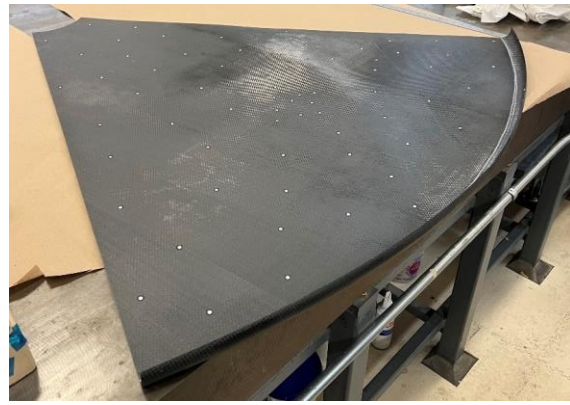
1/6 Gore of 3 meter-paraboloid dish was fabricated for folding test
